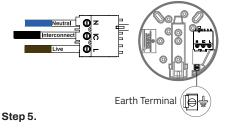
Connect the wires to the terminal block; L: Live (Brown), N: Neutral (Blue), IC: Interconnect (UK/Black) or (ROI/White)
